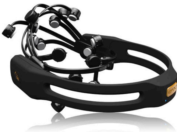
Figure 4: The Emotiv EPOC headset
