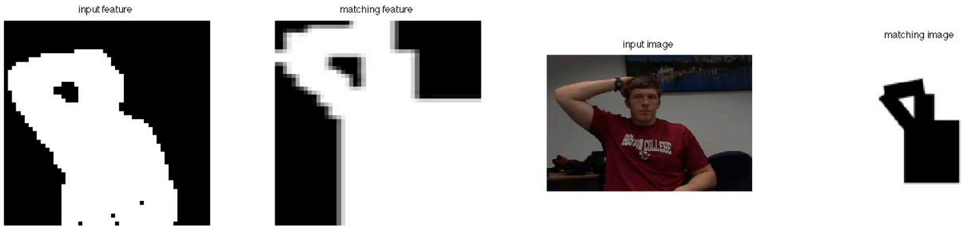
Figure 14 – Example successful matches using the stick figure dataset. From left to right the images represent: an input feature, the matching feature pulled from a locality sensitive hash lookup, the input frame of video, the pose information matching the feature pulled from the database.
