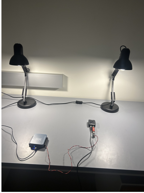
Figure 2.7 Sampling with Sensor 65cm from Bulb-A
